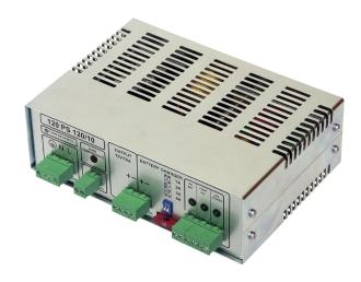
If the voltage failure is long time, the voltage on accumulator declines gradually. The decline under 11V (22 V) value with turn off LED diodes and turn on the U BAT 11V. If the voltage failure lasts further and there is danger of damage the accumulator with deep discharge, the accumulator is disconnected and the security system is not powered.
